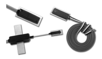
Micro-Measurements Sealed Weldable Strain Gages are specially designed for spot welding to structures and components. They are ideally used for applications where test or environmental conditions preclude clamping and curing an adhesively bonded gage installation. These gages
