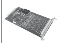
Model 7100-8-LVDT is used to perform signal conditioning, polarity demodulation and AC excitation for Transformer-type transducers.
