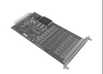
Model 7100-8-HL High Level Input Card is used to perform signal conditioning and excitation for high level (±10V) inputs.
