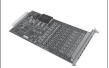
Model 7100-8-SG Strain Gage Input Cards accomplish bridge excitation, bridge completion, shunt calibration, and signal conditioning for eight quarter, half, and full bridges.
