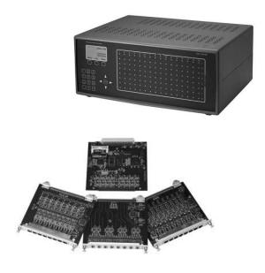
Scan rates up to 2048 samples per second are available for simultaneous reading of all sensor inputs. A combination of analog and flexible Finite Impulse Response (FIR) filters are available to provide adequate anti-alias filtering at all scanning rates. Each sensor card has high-capacity nonvolatile data storage capability. Electronically selectable bridge completion resistors allow the user to choose between 120-, 350-, and 1000-ohm strain gages through software selection.
