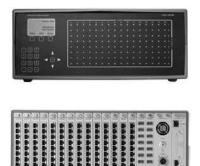
The purpose of the Model 7000-128-SM Scanner is to house and retain the acquisition cards, regulate power to the cards, establish and maintain communication between the Ethernet interface and the input cards, synchronize the analog-to-digital converters in the system, and provide visual status information to the operator.
