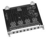
The Model 7003-8-TC Thermocouple Input Card is used in conjunction with the Model 7003-8-A-I Analog Input Card to perform signal conditioning and cold-junction compensation for thermocouple types J, K, T, E, N, R, S, and B.
