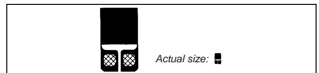
Fig. 4.7 - 5000ohm transducer strain gage with copper soldering pads on gage tabs.
