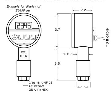
\* Models JHB, JHE, JHR, JHX, JHV No cable for battery powered Model JHW
