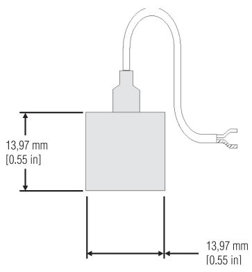
Model MA23 Accelerometer
