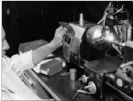
Welding technology for hermetic sealing of transducers.
