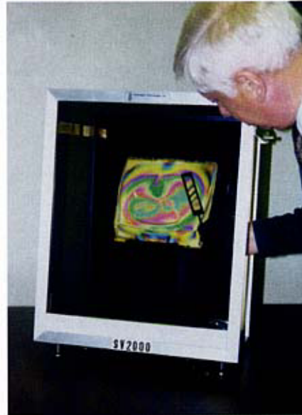
Figure 2. Residual strains become visible using the SV-2000 Strain Viewer and can be quantified with an optional Strainoptic LWC-100 Compensator
