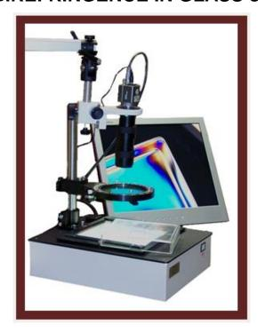
The PS-100-DIGIVIDEO Polarimeter system is the ideal solution for measuring <u>and digitally storing</u> residual stress or birefringence information from a wide variety of applications and industries. Its uses range from simple inspection and interpretation of photoelastic colors to precise quantitative measurements using analyzer rotation or compensation techniques.
